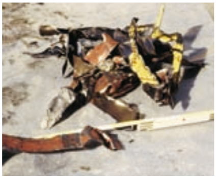
Shredded barrel material pumped with sludge
